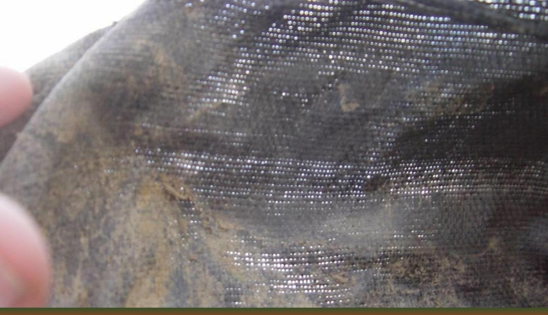
Woven filter, not blinded, sunshine visible through weave. Woven filters can sometimes be blinded from either the river or bank side
