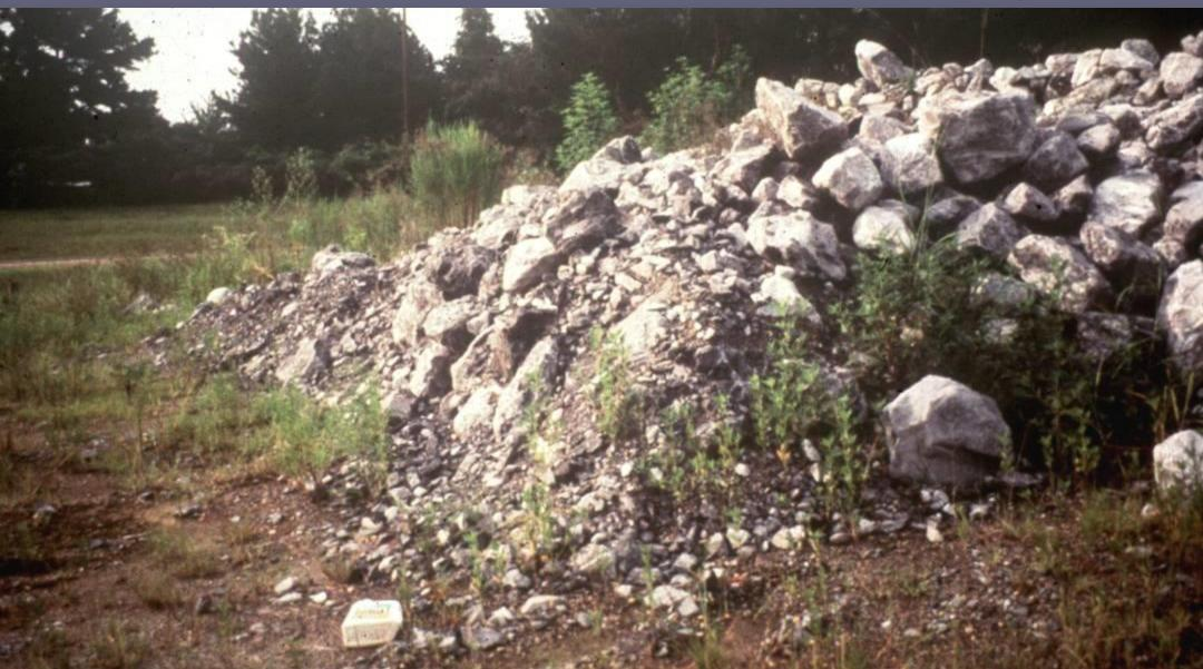
Analyze gradation, amount of "fines", look at pile side slopes (flatter is better). Climb the pile, if it moves that is the stone you need. This is well graded stone, note flat angle of pile
