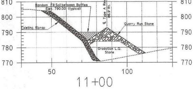
**LPSTP Cross-sections.** Top bank = el. 806Q-2 flow = el. 803**LPSTP crest = 793 Designed to be** overtopped 13 days/yr. **Core section of LPSTP** was built of a less expensive stone, while quarry run stone was used for all exposed surfaces
