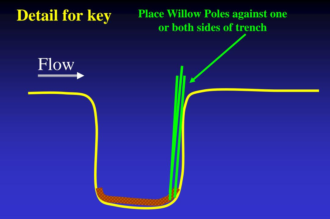
**Construction** 9/19/2006. **Digging a mid**project key perpendicular to the bank. Some veg (willow poles) in place
