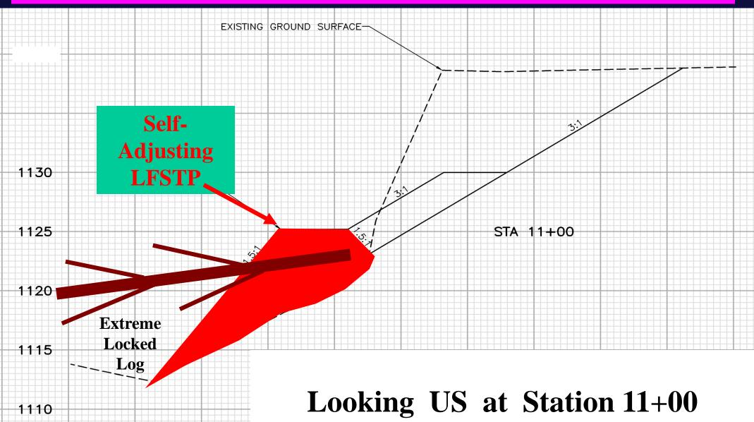
LONGITUDINAL FILL STONE TOE PROTECTION WITH INTEGRATED EXTREME LOCKED LOGS (Fuzzy Locked Log shown next)
