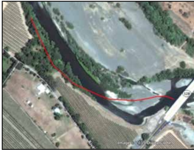
Google view taken pre-project 2010, Red line is toe of old bank which was protected with riprap until 2003. Bank migrated over 60-feet in 7 years.
